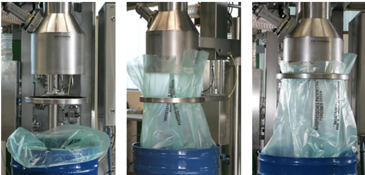
pressure, which is needed for shaping of the container, must be adapted to the thickness of the interior bag. If the pressure is too small it will not be enough for an ideal shaping and if the pressure is too high it can destroy the container.
